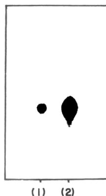
FIGURE 6: Identification of B-T-1 with synthetic isoleucylprolyl-proline by thin-layer chromatography: solvent, 1-butanol-acetic acid-H 2 O (3:1:1, v/v). Peptides were located with peptide reagent: (1) B-T-1; (2) Ile-Pro-Pro.
